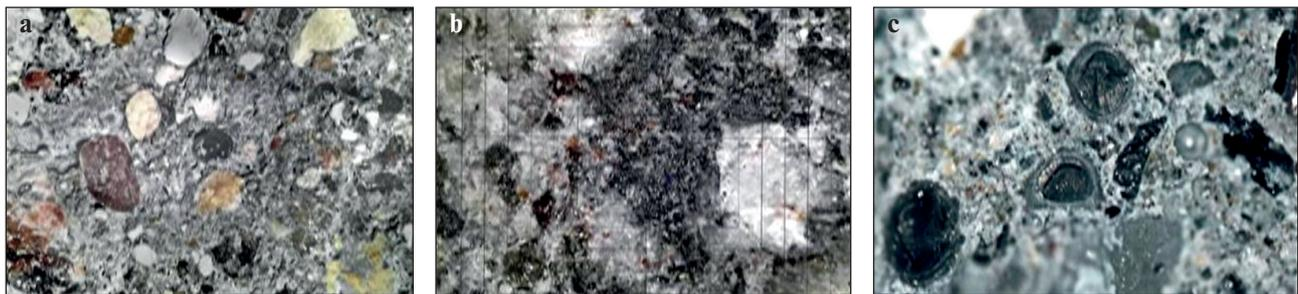
Fig. 7. Microstructure of polymer concrete samples: a – based on FA monomer; b – based on FD resin; c – based on FOD resin
